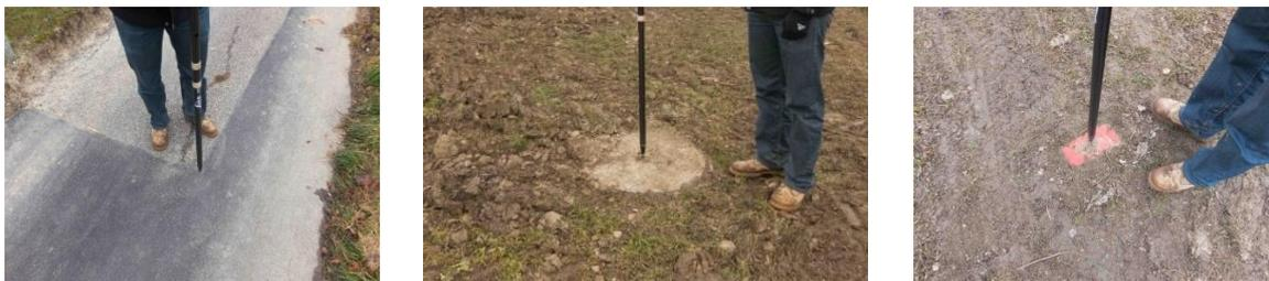
Figure 5. Examples of GCP (artificial and natural).
